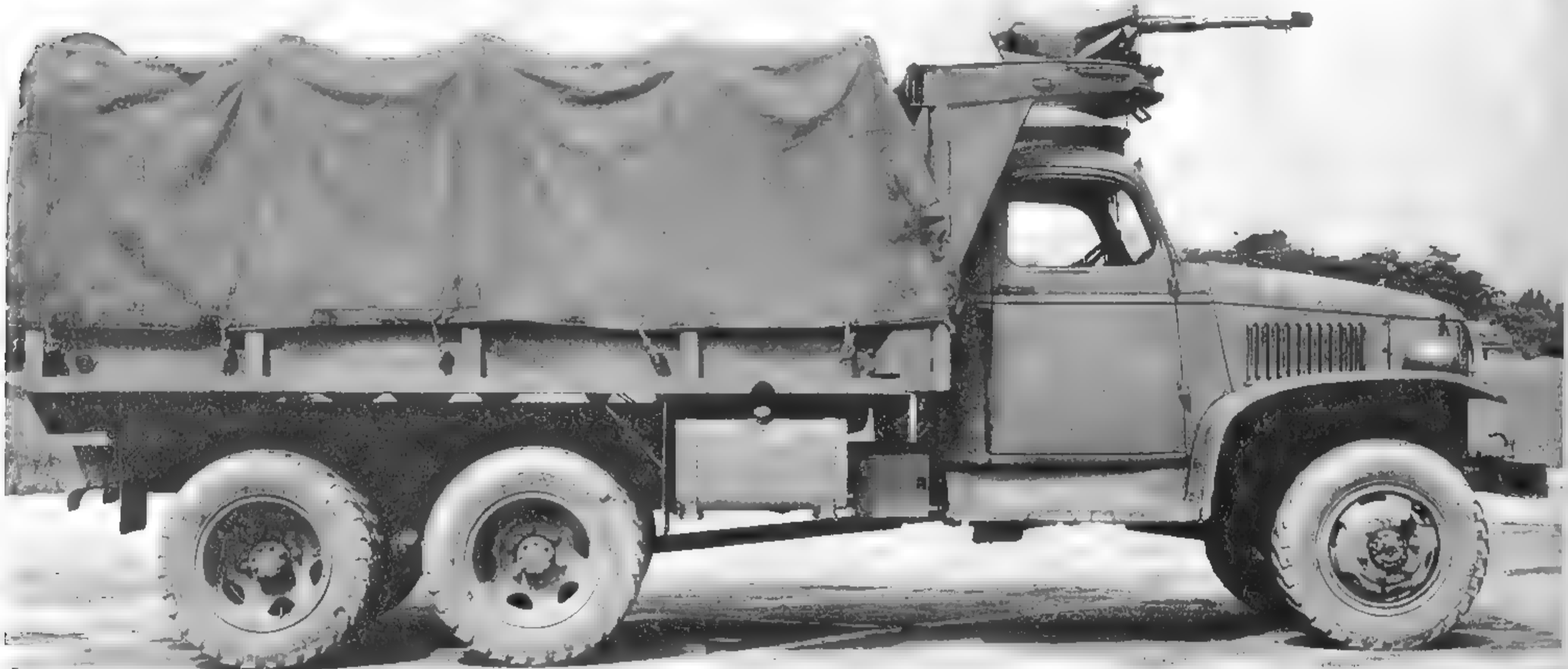
The fuel tanks on the long-wheelbase CCKW-353 trucks were mounted beneath the bed on the passenger's side. This closed-cab truck sports an M32 ring mount and M2HB .50-caliber machine gun. (National Archives and Records Administration photo)
